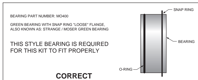
Figure 2. Loose Fit Bearing Configuration
