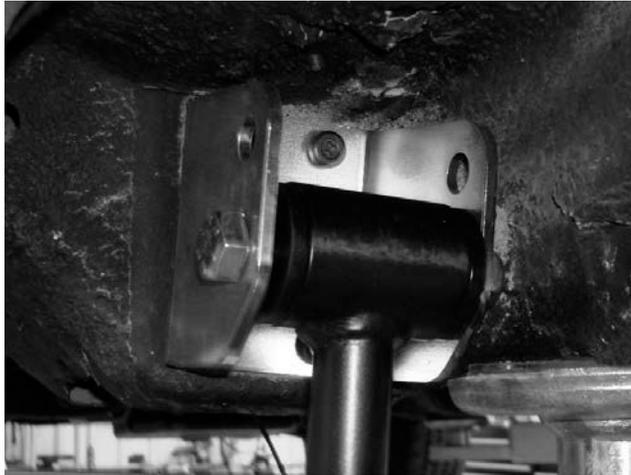
9- With a suitable jack, or jack stands, place the axle under the car and attach the lower links to the axle brackets. Put the link in the upper hole on the axle bracket.
