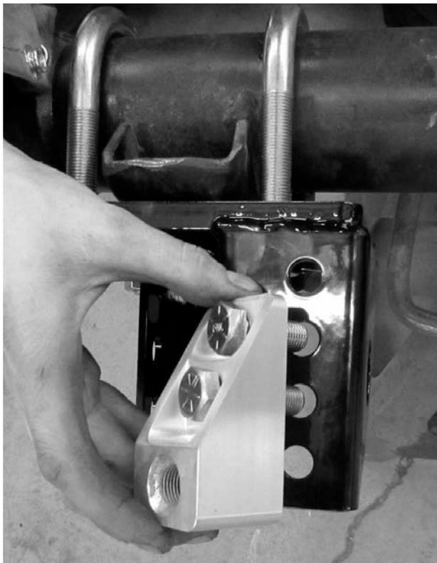
8- The lower links can now be installed in the car, along with the axle. Bolt the lower link first to the included new front hanger, then bolt it into the factory leaf spring location in the car. Make sure the grease fitting in the link is pointing down so you can access it later. Put the link in the lower hole in this front bracket.
