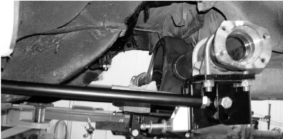
10- The axle now needs to be properly located in order to weld the upper link bar mounts onto the axle in the correct location. If you also purchased the fully welded housing from RMS, this step can be skipped.
