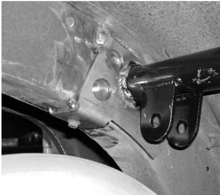
way around the side plates. The 1" holes in the side plates should also be welded in for maximum strength.
