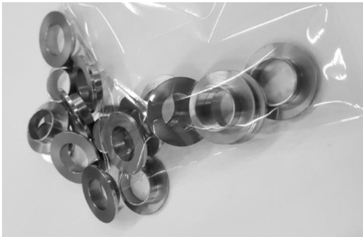
6- These spacers correct the width and hole size to properly fit the new links. Install the spacers from the outside of the front hanger bracket as shown –
