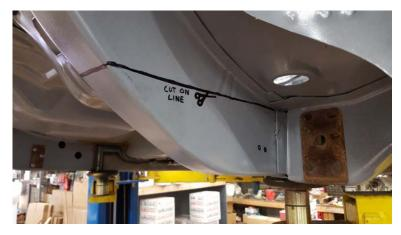
This is the cut line. Cut out this entire bottom section of frame rail. You do not need to reinforce the car before doing this, and it's safe to do on a lift without the car flexing.
