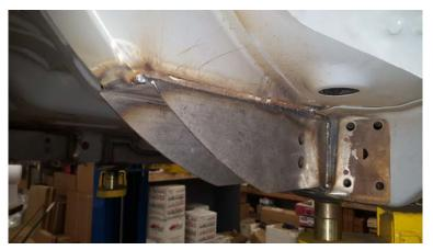
Fully weld around the entire perimeter of the boxes, up the front edges and across under the bottom.
