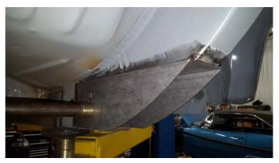
Notice the boxes fit tightly for a good weld, and now recreate the bottom shape of the frame rail.
