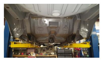
Complete. You can now trust that you have square and parallel suspension mounts. Also note that the suspension loads are now directly inline with the frame rails and frame connectors for a good strong platform.
