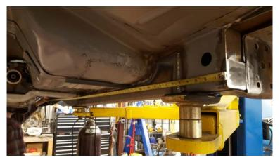
Next measure forward from your cut line to a reliable place on the car, such as the transmission crossmember or front suspension subframe. The factory mounts are often not the same. Note which side is further back in the car. Factory errors can be ¼" from one side to the other. Do Not Trust the original mounting pads to be square!
