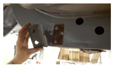
Note on the driver side you need to remove the parking brake cable bracket so you can put it back on later if desired.
