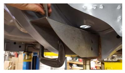
First, hold the box against the frame, tight forward against the leaf spring mounting pad, and mark the frame with the top surface of the box.
