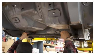
Hold the boxes in place, centered under the frame rails. Remember which one was further back in the car – tack this one in place. Then move to the other box and move it forward slightly to nearly match the distance of the first one. The difference could be up to ¼", so be careful to only move it so much that you can still weld the gap in front of the box.
