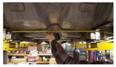
First measure the width across the rails, center to center. You will preset the boxes to this width before welding.
