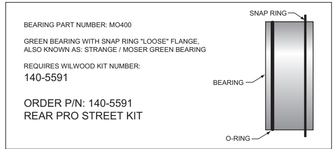
Figure 2. Loose Fit Flange Bearing Configuration
