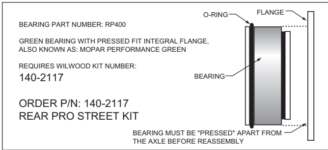
Figure 1. Press Fit Flange Bearing Configuration
